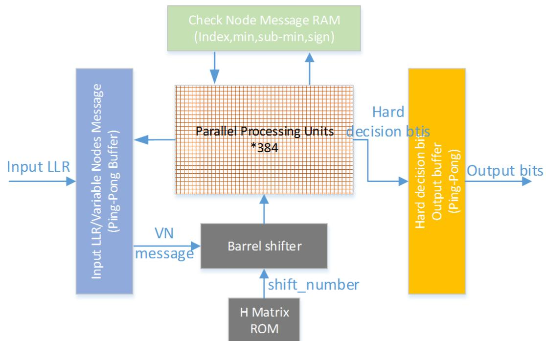
Figure 1: LDPC Decoder Core Block Diagram
